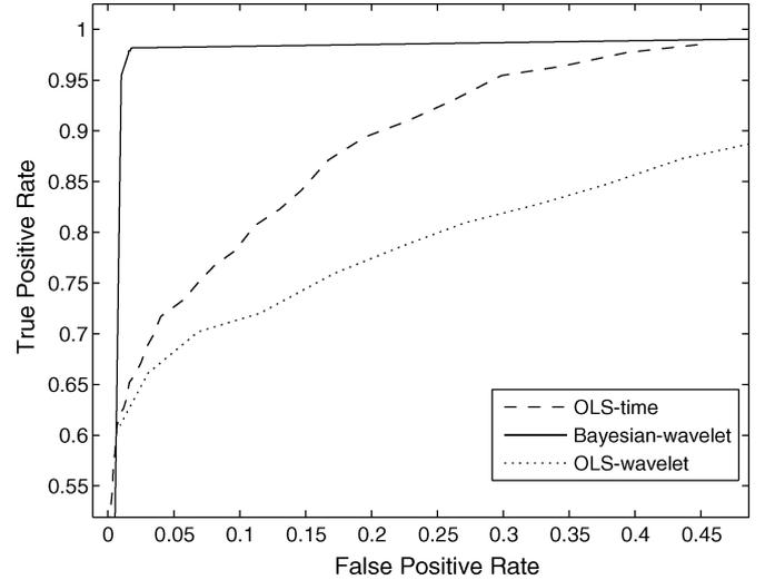
Fig. 5. ROC curves of OLS (in time domain and wavelet domain) and Bayesian (after DWT) methods for simulated fMRI data corrupted with fBm noises.
