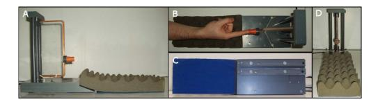
**Fig. 1** Photographs of the force coil. **a** Side elevation showing coil, finger guard and wrist rest. **b** Top elevation showing position of wrist on rest, and with restoring bands and marked angles visible. **c** Bottom elevation showing tracks for 3T and 7T magnets. **d** Front elevation showing supports on either side and finger guard.
