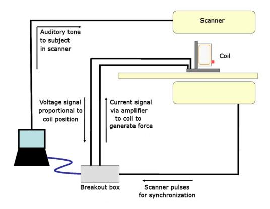
**Fig. 2** Experimental setup and sample data. A laptop running MATLAB controls the session. To time the force sequences, pulses from the scanner are read by a digital input on the breakout box and recorded using a NI-DAQ card. The laptop sends a tone to the subject in the scanner at the start of each force sequence and analogue voltages are sent to the coil via a current amplifier to produce these forces. During the sequence the position of the potentiometer on the coil is recorded.
