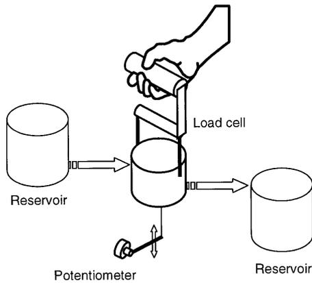
**Fig. 1** The experimental arrangement. The two water reservoirs were connected by flexible tubes to the central container, allowing silent flow of water in or out. The load on the handle was recorded, and the height of the container was measured by a potentiometer linked to the container by a lever
