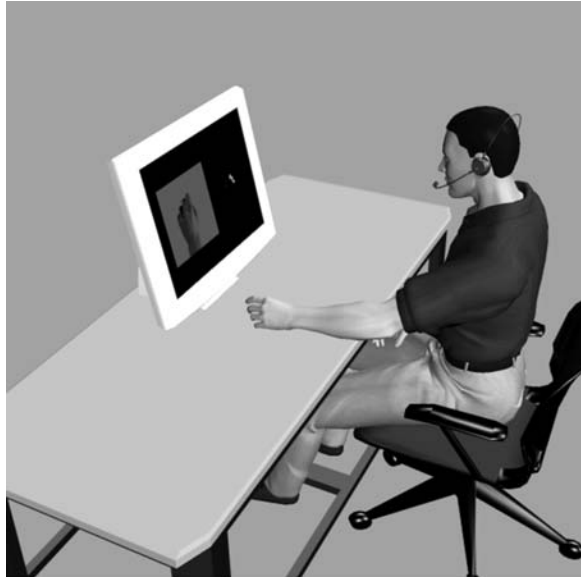
181 Fig. 1 Top panel: 182 Experimental setup for the 183 behavioral experiments. The 184 participant moves his or her 185 hand in time with the visual 186 metronome on the right of 187 the screen, and responds 188 vocally to target stimuli via 189 the microphone. Bottom 190 panel: Example display 191 screen, showing one hand 192 picture from the visual series 193 on the left of the display, 194 and the visual metronome on the 195 right of the display (metronome not to scale)
