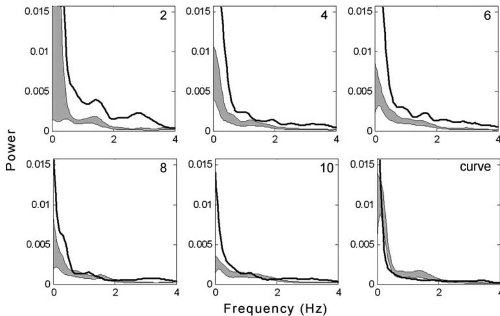
**Fig. 5** Mean power spectra calculated for tracing around the curved template shapes. Control data are indicated by the grey zone,  $\pm 1$  SEM around the group mean. The average power spectrum for subject IW is shown by the heavy black lines. Note the
